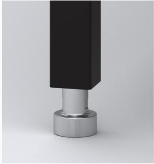
Place the kitchen in position as shown in the plan previously sent for utility arrangements. Adjust the feet with the 16 wrench. The kitchen should be adjusted to a height of 90 cm. The adjustment allows a range of +/- 1 cm
