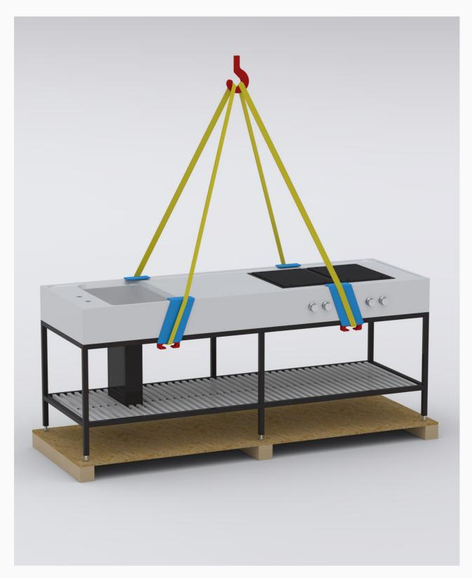
Sling the kitchen with lifting straps by passing through the appropriate position handles and taking care to place the protective material between the straps and the concrete top. For enclosed kitchens, the handles are at the bottom.
