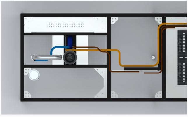
Install the tap and mixer following the manufacturer's instructions, connect hot and cold water via hoses placed between the concrete top and the thickness of the frame reaching the tunnel for the final connection.
