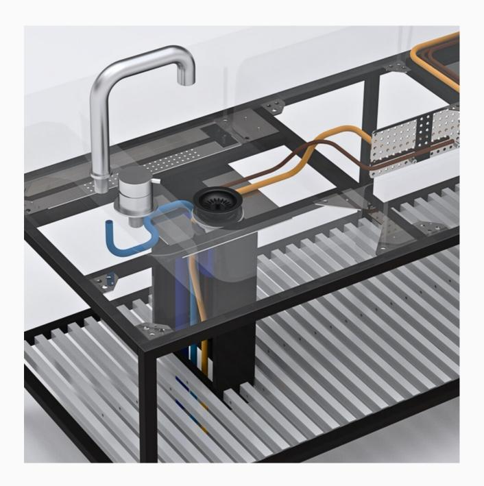
Install the induction/gas cooktops following the manufacturer's instructions by feeding them through electric cables (brown tube in the picture) and gas tube (yellow tube in the picture) from the tunnel to the wiring plate located vertically in the under-top compartment. The tubes should run in the frame space, adjacent to the concrete top.
