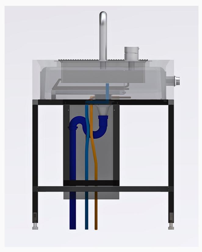
Install the drain pipe with the siphon (dark blue tube in the image). Check the connections and perform a drain test before closing the side panel.
